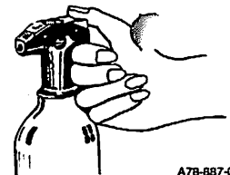
FIGURE 5: Aim Nozzle and Squeeze Lever to Discharge Powder
